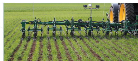
Figure 2| Interrow hoeing with automated steering using vision techniques.
