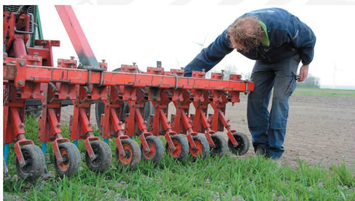
Figure 1| Setting the right cultivation depth for mechanical weeding is key to avoid germination of new weeds
