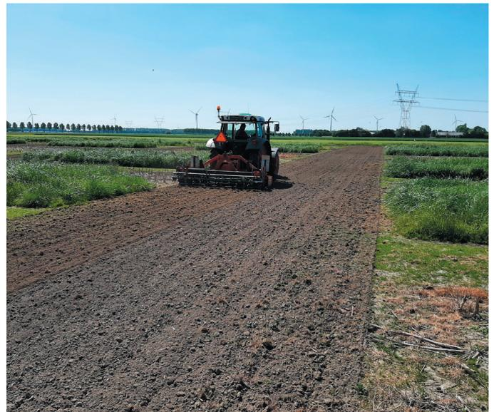
Figure 2 | Shallow rotary tillage operation after ploughing to prepare the seedbed and to control emerging seedlings of weeds.
