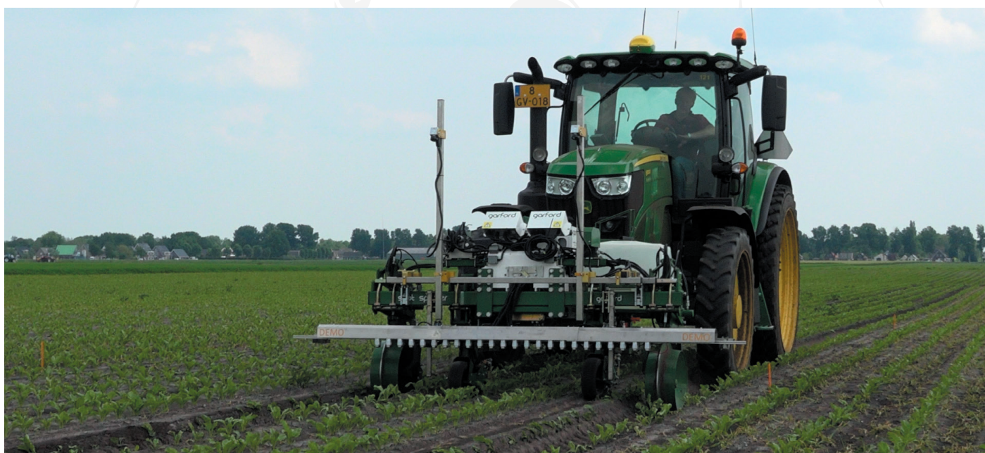
Figure 1| Scouting through identification with algorithms combined with spot spraying to terminate weeds.
