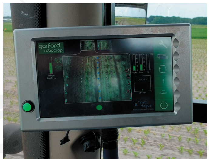
Figure 1 | The Garford robocrop is an in-row weeder that locates individual crop plants based on video image analysis.
